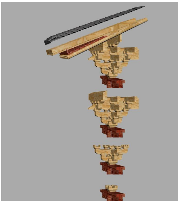
Figure 5: Compiled screenshots of an Autodesk Maya rendering of dougong. Using animation, virtual stacking of dougong components are able to demonstrate the constructional formation (Lai, 2018).
