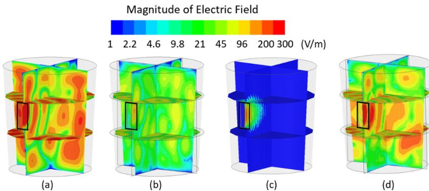
**Fig.1.** Simulated magnitude of the electric field, with 1W incident power at 2.45 GHz, inside cavities completely filled with (a) LDPE and Polystyrene,  $\epsilon_r$  of 2.25,  $\tan\delta$  of .0003, thermal conductivity of .28 W/m°C, density of 950 kg/m<sup>3</sup> and specific heat of 2300 J/kg°C, (b)
