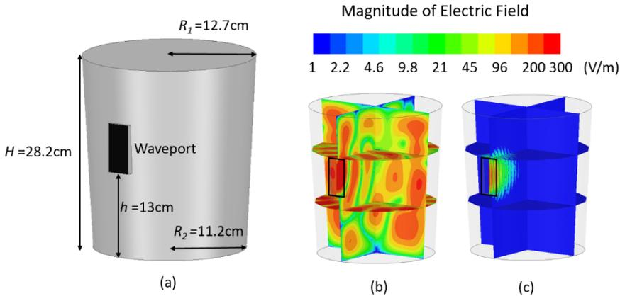
**Fig 2.** Simulated magnitude of the electric field for a single waveguide port excitation of a cavity completely filled with various materials. (a) Simulated cavity with dimensions labeled. (b) Cavity filled with food mixture  $\epsilon_r = 42$  and  $\tan\delta = .3$ , and (c) Cavity filled with LDPE and polystyrene  $\epsilon_r = 2.25$  and  $\tan\delta = .0003$ . The field value is normalized to a 1W incident power at 2.45 GHz on waveguide port.
