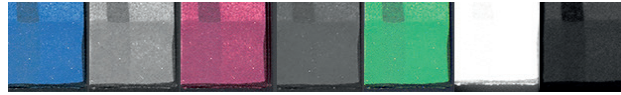
Figure 5 | Egyptian blue pigment pattern, from left to right VIS-R_VIS, IR-R_IR, IRFC, UV-R_UV_365, UVFC, IR-L_VIS and IR-L_UV_365. Pigment Samples made by Roland Lenz, ABK Stuttgart. Source A. Keller.
