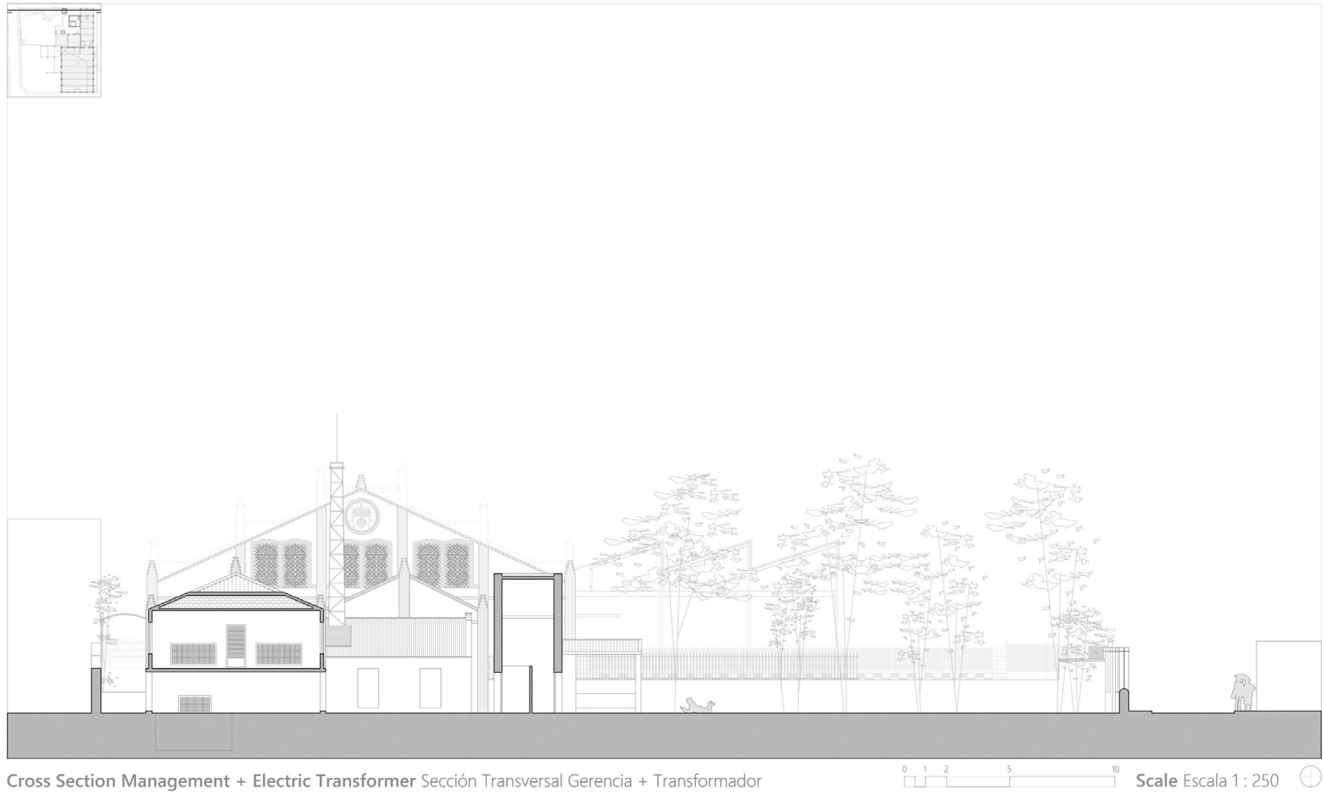
Fig 14. Taller dels Canets (former San Antonio wooden carriage factory), Beneixama (Alicante, Spain), April 2021. Current state drawing of cross section made by the two furthest volumes, the management and the electric transformer, raised on the wall. (Ortín Molina, S.; Ortín Molina, M. A., measurements by hand and drawing in AutoCad).
