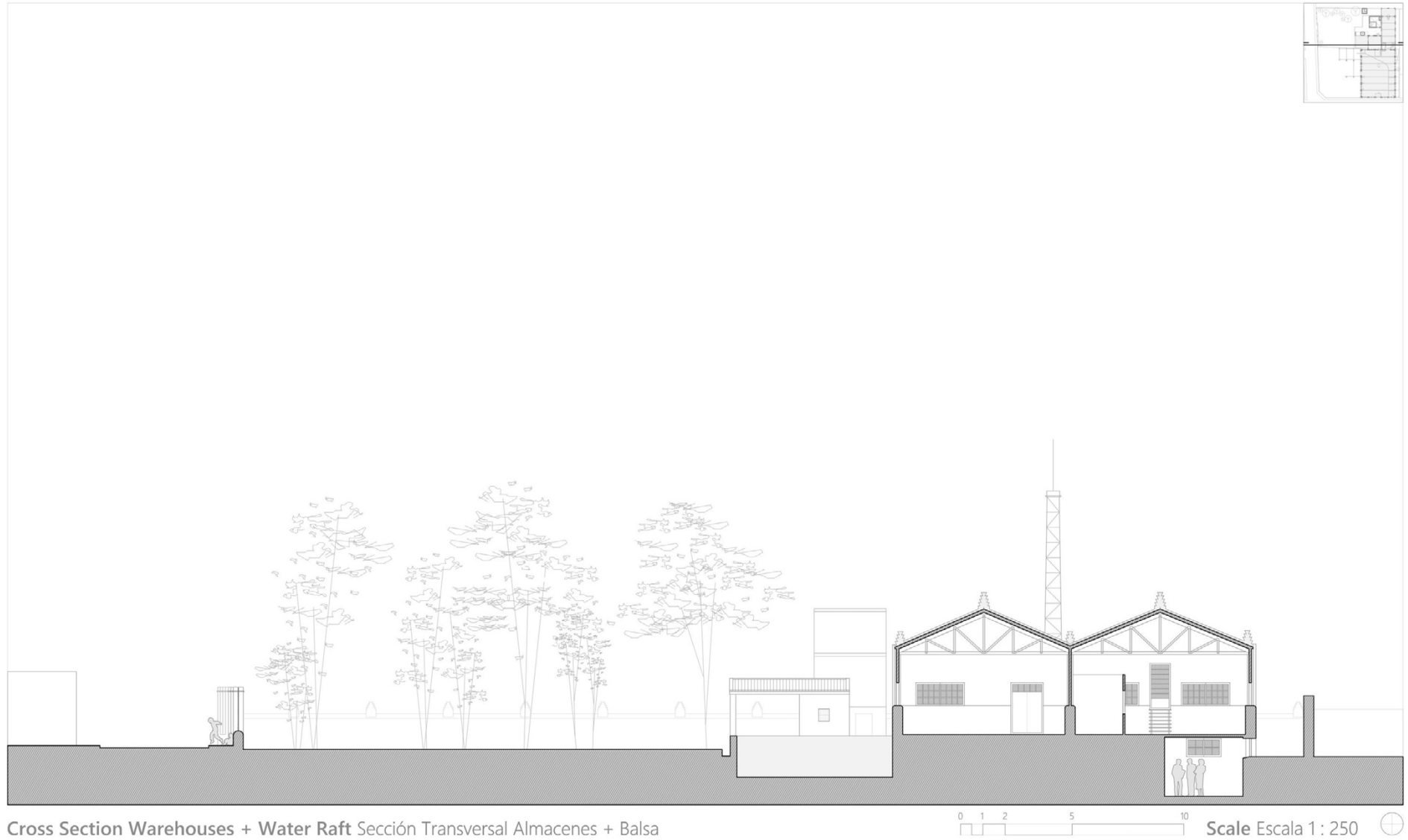
Fig 12. Taller dels Canets (former San Antonio wooden carriage factory), Beneixama (Alicante, Spain), April 2021. Current state drawing of cross section made by the attached warehouses and the wáter raft. The semi-buried spaces can also be seen. (Ortin Molina, S.; Ortin Molina, M. A., measurements by hand and drawing in AutoCad).
