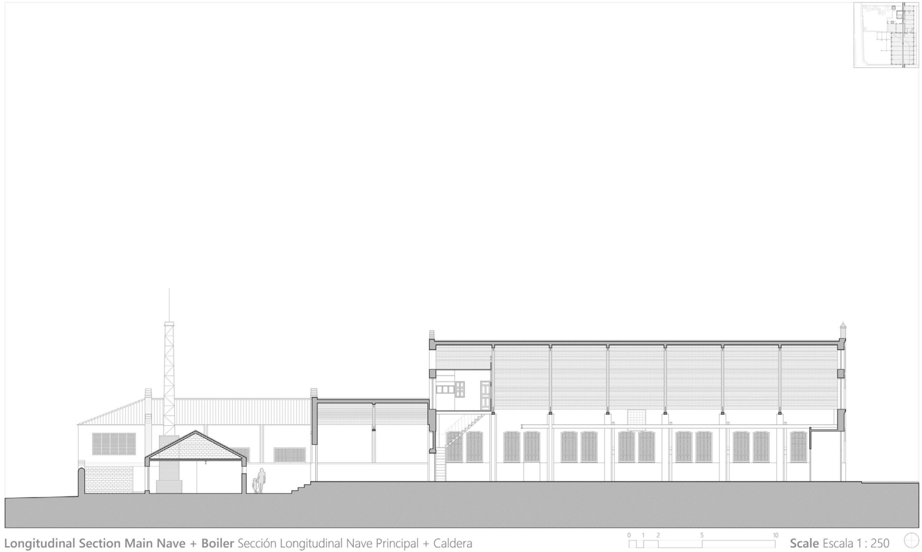
Fig 16. Taller dels Canets (former San Antonio wooden carriage factory), Beneixama (Alicante, Spain), April 2021. Current state drawing of longitudinal section made through the middle of the nave. The difference in height existing in the plot appear. (Ortín Molina, S.; Ortín Molina, M. A., measurements by hand and drawing in AutoCad).
