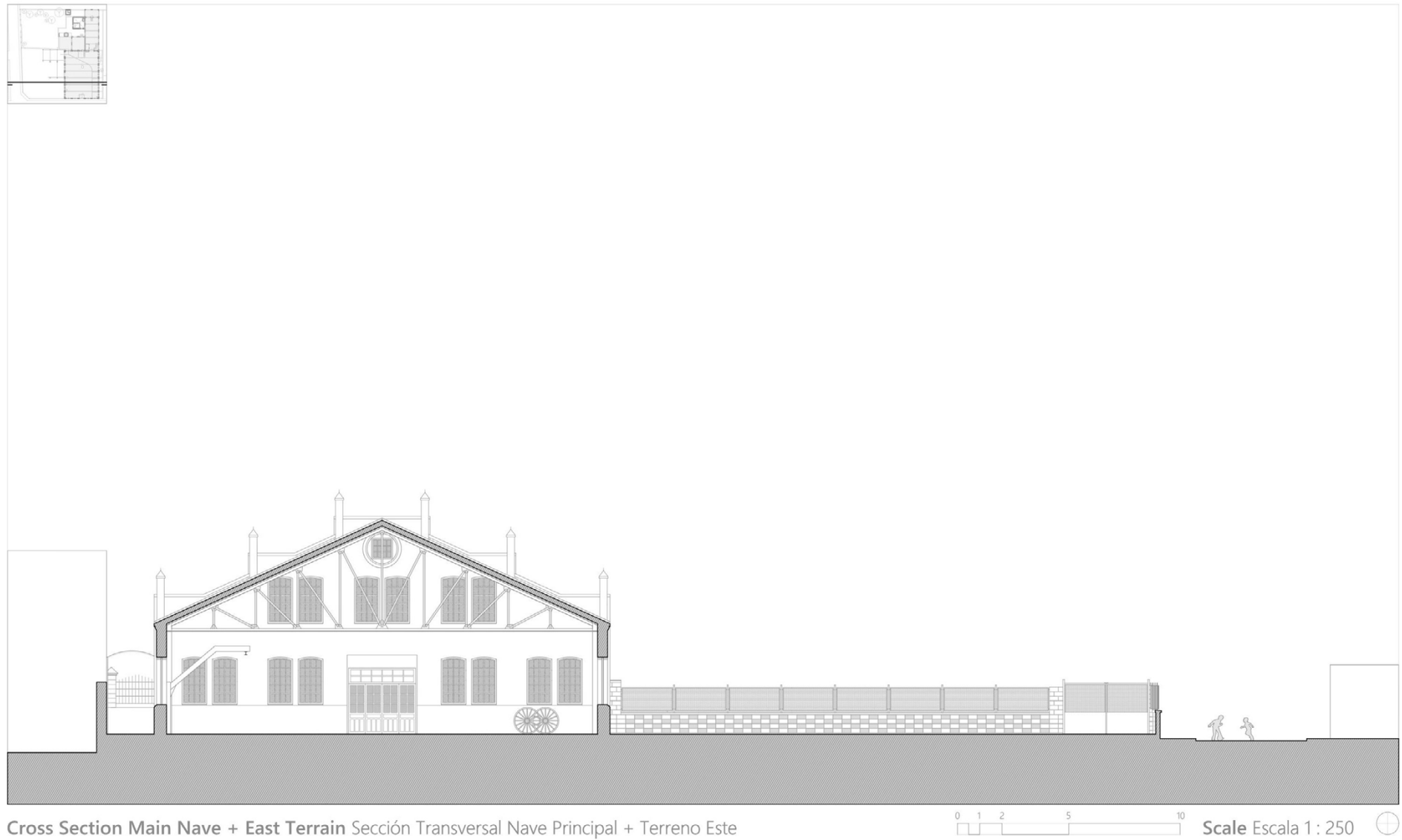
Fig 10. Taller dels Canets (former San Antonio wooden carriage factory), Beneixama (Alicante, Spain), April 2021. Current state drawing of cross section made by the third north span of the main nave. The background fences are shown in their magnitude. (Ortín Molina, S.; Ortín Molina, M. A., measurements by hand and drawing in AutoCad).
