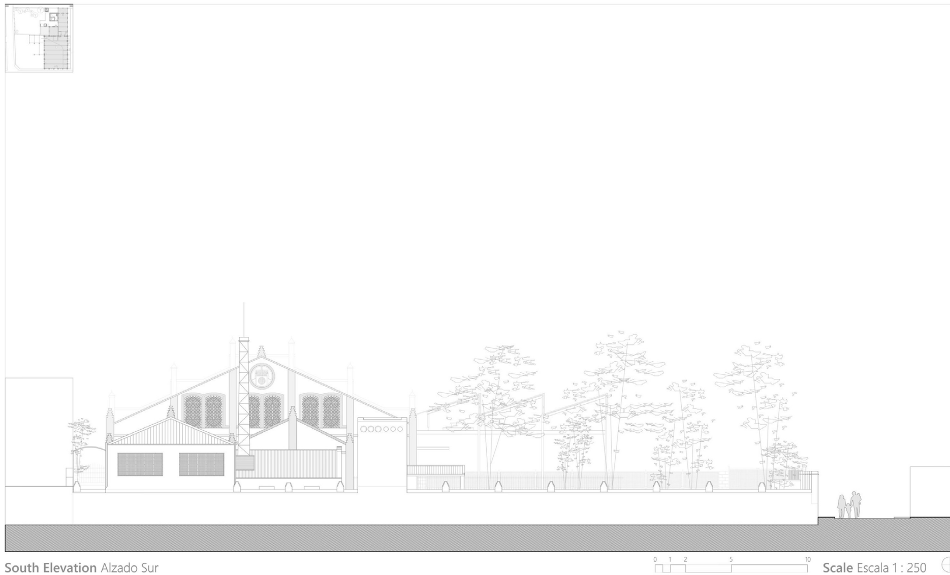
Fig 9. Taller dels Canets (former San Antonio wooden carriage factory), Beneixama (Alicante, Spain), April 2021. Current state drawing of South elevation. The rear façade, more heterogeneous, shows the different volumes of the factory over the long wall. (Ortin Molina, S.; Ortin Molina, M. A., measurements by hand and drawing in AutoCad).
