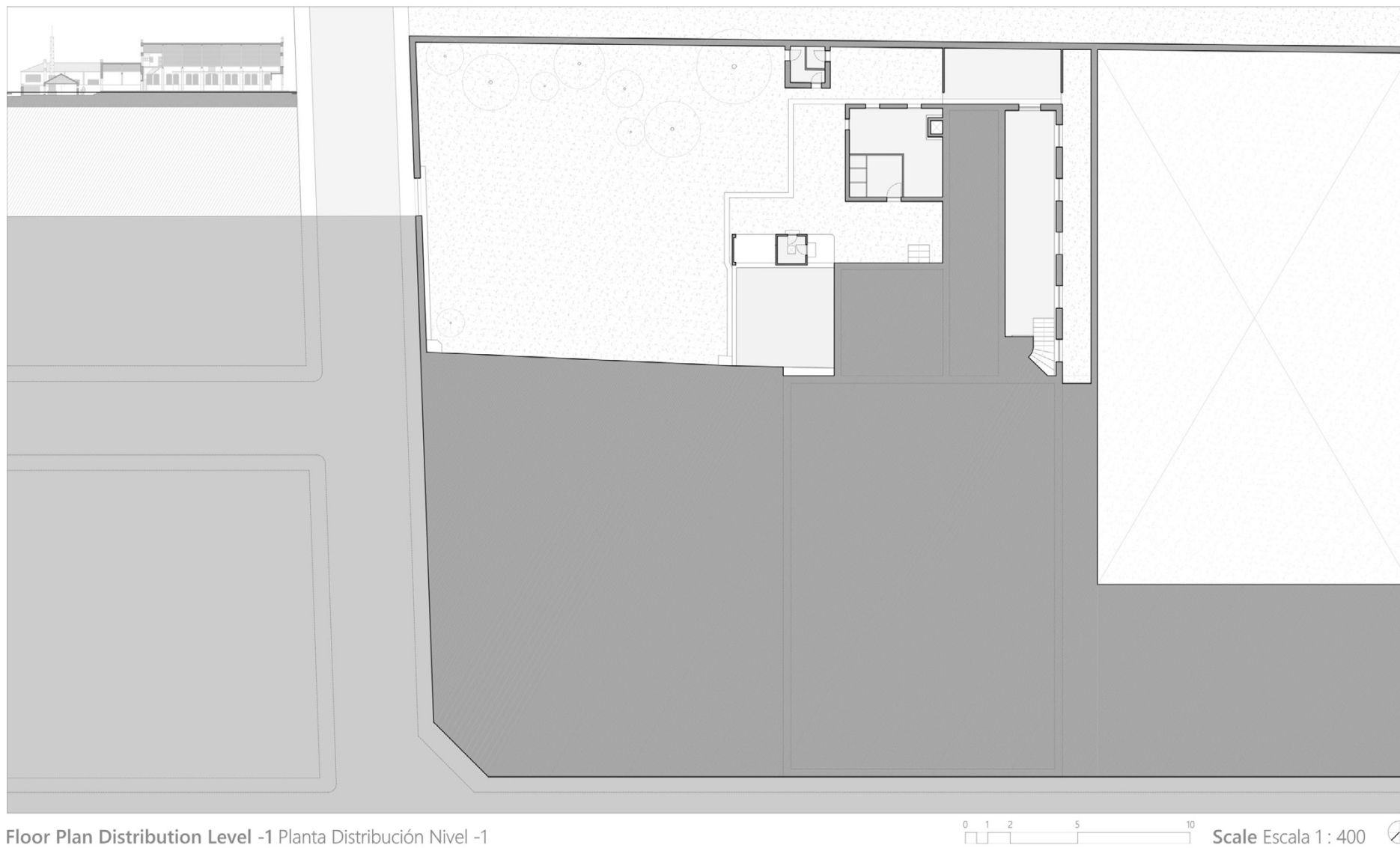
Fig 3. Taller dels Canets (former San Antonio wooden carriage factory), Beneixama (Alicante, Spain), April 2021. Current state drawing of basement floor distribution plant, destined to underground warehouse, boiler, chimney, electric transformer and well. (Ortín Molina, S.; Ortín Molina, M. A., measurements by hand and drawing in AutoCad).
