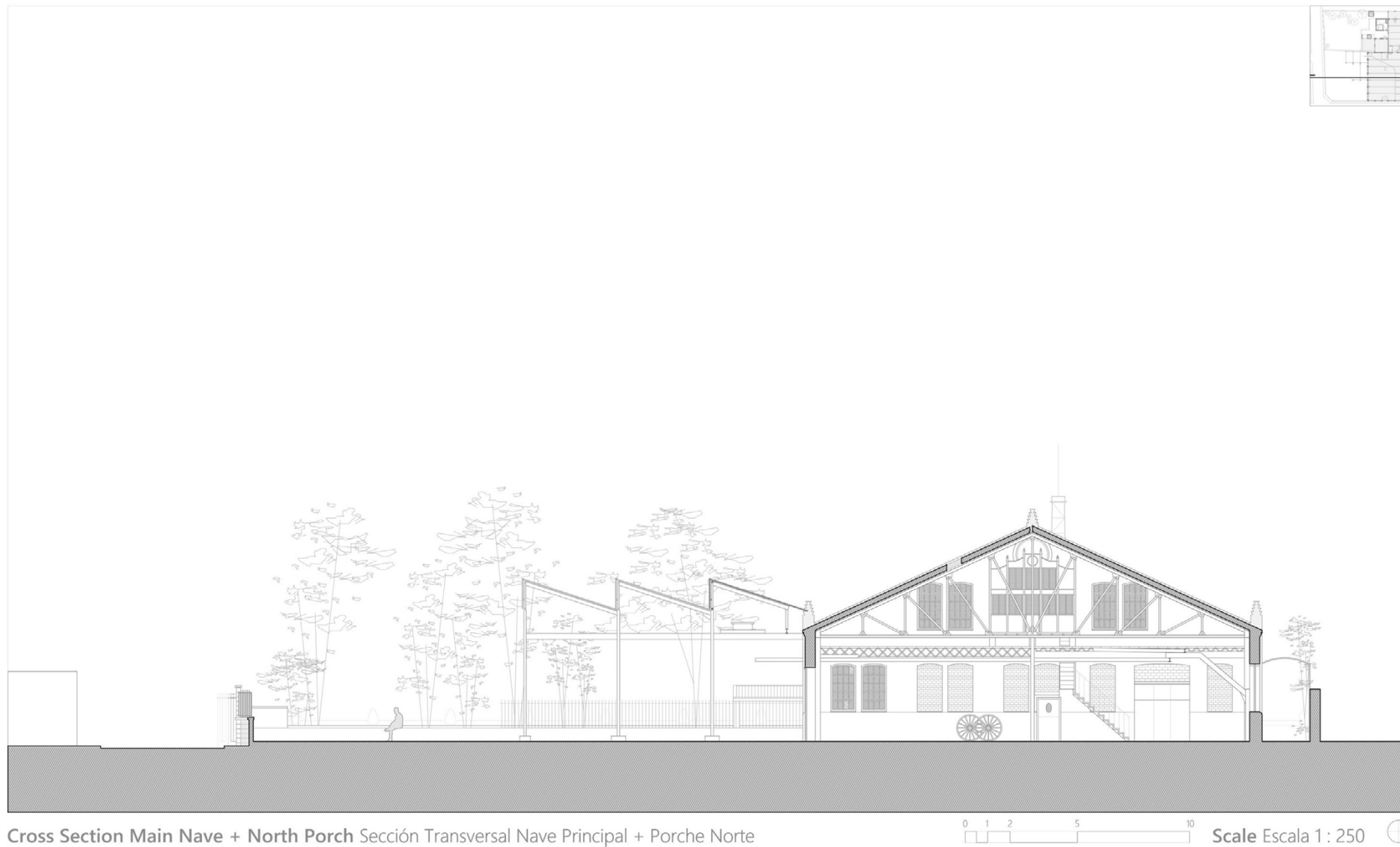
Fig 11. Taller dels Canets (former San Antonio wooden carriage factory), Beneixama (Alicante, Spain), April 2021. Current state drawing of cross section made by the middle of the nave. In this span between trusses is the large open crack in the roof. (Ortin Molina, S.; Ortin Molina, M. A., measurements by hand and drawing in AutoCad).
