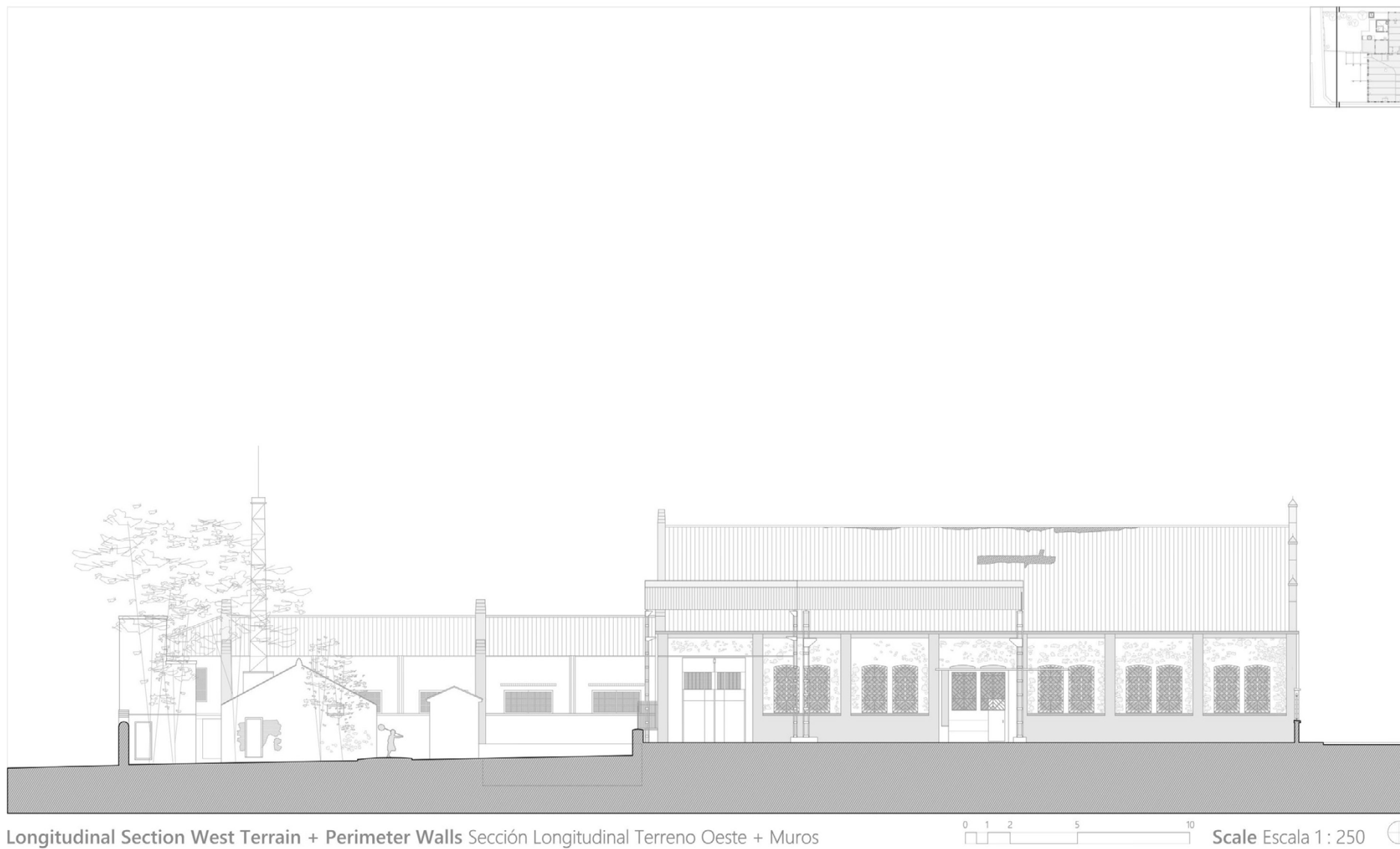
Fig 15. Taller dels Canets (former San Antonio wooden carriage factory), Beneixama (Alicante, Spain), April 2021. Current state drawing of longitudinal section made by the east terrain. The break in the modulation caused by the two doors can be seen. (Ortin Molina, S.; Ortin Molina, M. A., measurements by hand and drawing in AutoCad).
