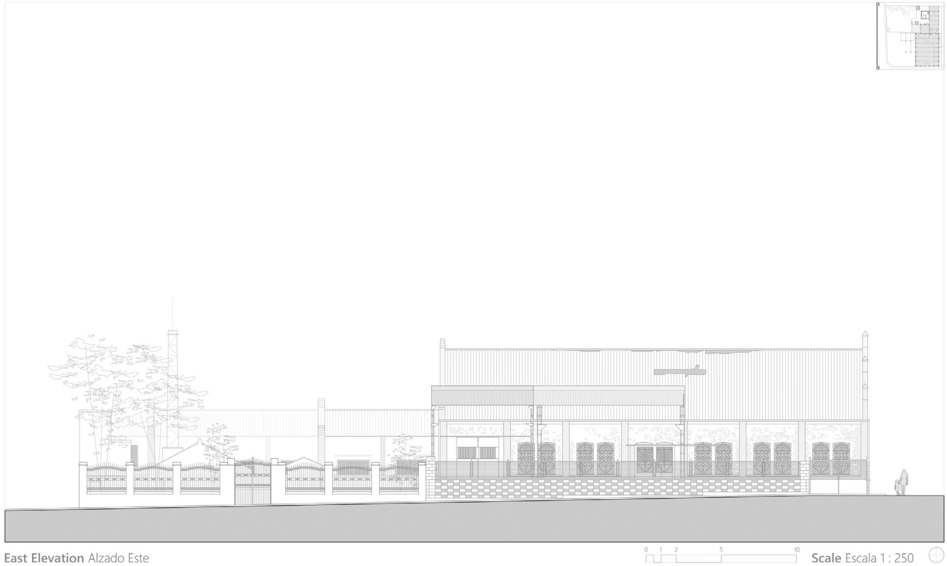
Fig 8. Taller dels Canets (former San Antonio wooden carriage factory), Beneixama (Alicante, Spain), April 2021. Current state drawing of East elevation. The side façade of the factory shows the organic growth of the industrial área, over time and needs. (Ortin Molina, S.; Ortin Molina, M. A., measurements by hand and drawing in AutoCad).
