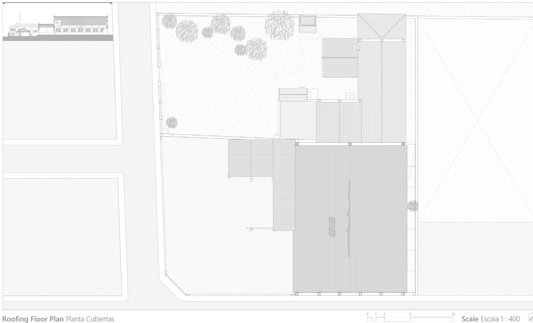
Fig 5. Taller dels Canets (former San Antonio wooden carriage factory), Beneixama (Alicante, Spain), April 2021. Current state drawing of roof plant. The open crack on the east side of the roof can be seen as a result of structural collapse of wooden joists. (Ortin Molina, S.; Ortin Molina, M. A., measurements by hand and drawing in AutoCad).
