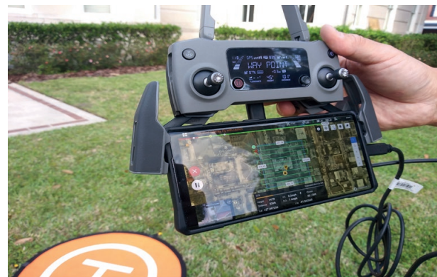
Fig. 11. The setup of a drone's remote control (RC) and a cell phone for pre-programmed flight over OPCCH. (Source: authors).
