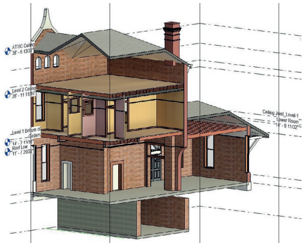
(c) A 3D view showing interior details with TLS point cloud turned off.
