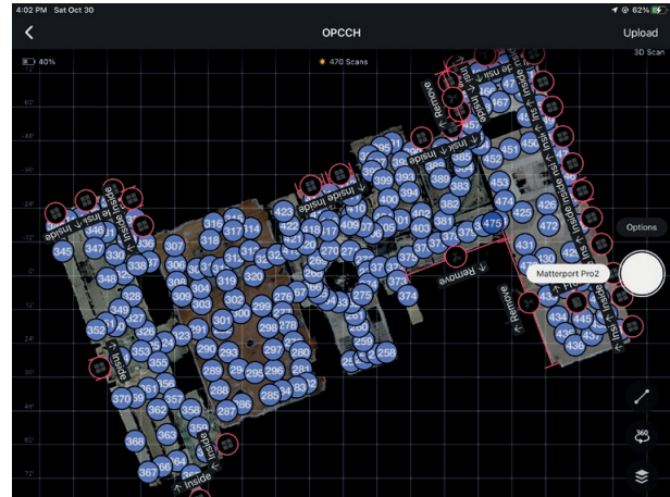
Fig. 10. The locations of the Matterport scans on the first floor shown on an Apple iPad mini. (Source: authors).
