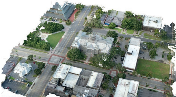
(c) 3D mesh generated from point cloud data.
