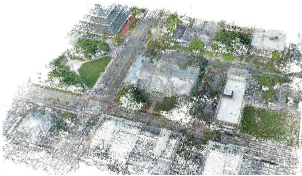
(b) Low-density 3D point cloud generated from aerial photos.
