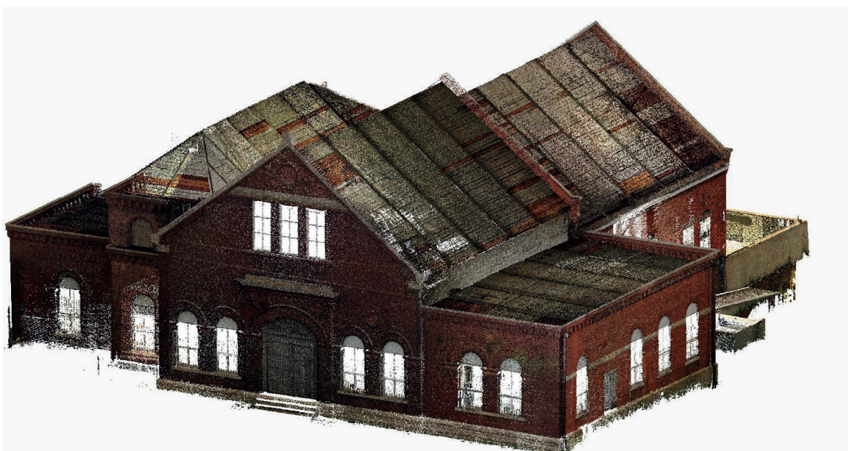
Fig. 2. A 3D colorized high-density point cloud captured using TLS. (Source: authors).
