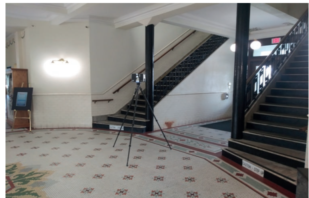
Fig. 7. A FARO Focus S-350 scanner scanning the interior of OPCC building. (Source: authors).
