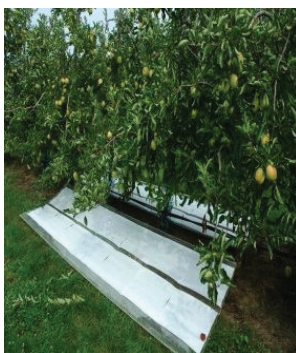
Figure 3. Deposit measurement on the soil with filter papers.
