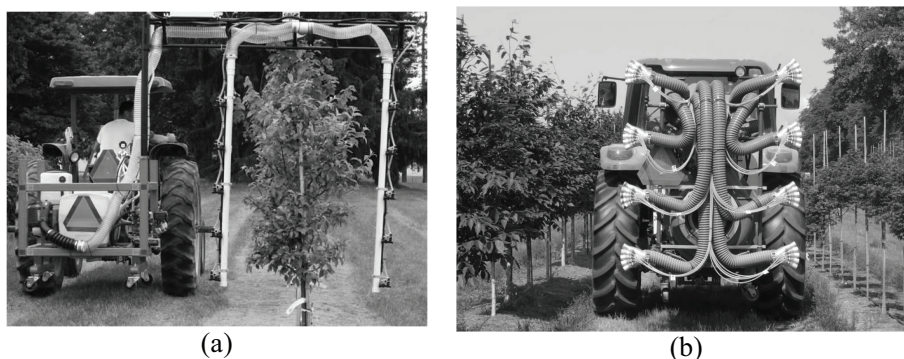
Figure 1. Two variable-rate precision sprayers developed for fruit and ornamental nursery crop applications: (a) hydraulic boom spraying system, (b) air-assisted spraying system.
