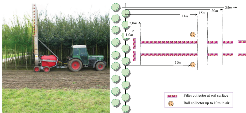
Figure 1. mast sprayer used in high nursery trees (left) and schematic lay-out of spray drift experiment
