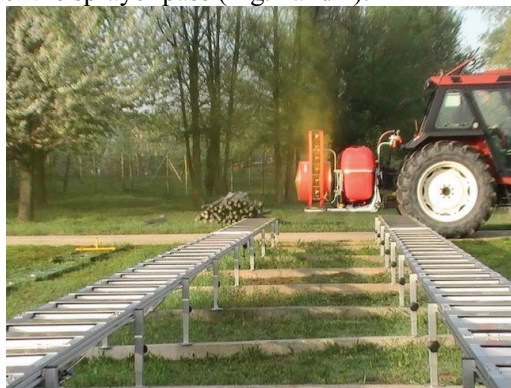
Figure 1. Test benches placed orthogonal to the sprayer pass in order to assess the spray fallout.
