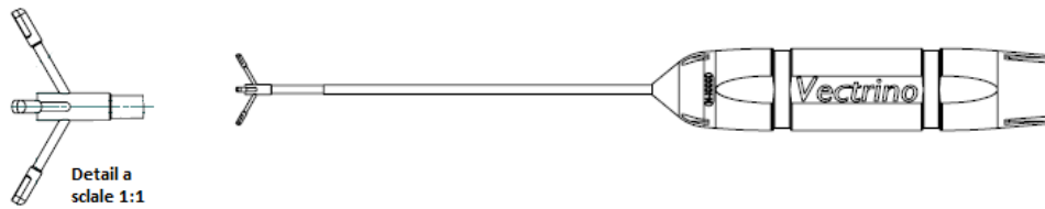
Figure 24. Vectrino 3D downlooking fixed stem and detail of this head.
