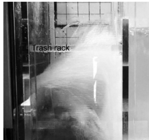
Figure 21. Jet while reopening of the intake gate.
