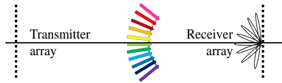
Figure 7-3: With linear arrays, data streams are mapped onto angles of arrivals
