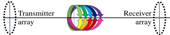
Figure 7-4: With circular arrays data streams are mapped onto vortices of various orbital angular momentums
