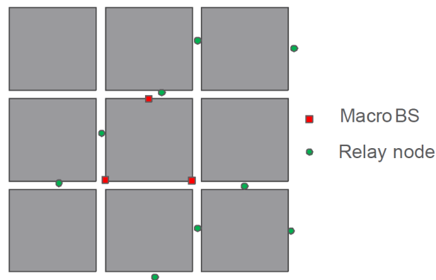
Figure 8-50: Deployment of macro stations and relays
