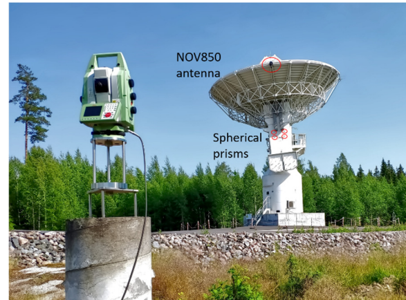
Figure 2. Simultaneous tachymeter and GPS local tie monitoring.
