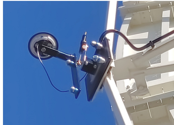
Figure 1. GNSS antenna on the left side of the VLBI-antenna with the compensator. The black Thorlabs plate was installed by the manufacturer of the VLBI telescope.
