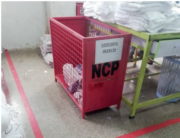
Figure 4: Non-Conforming product (NCP) area.
