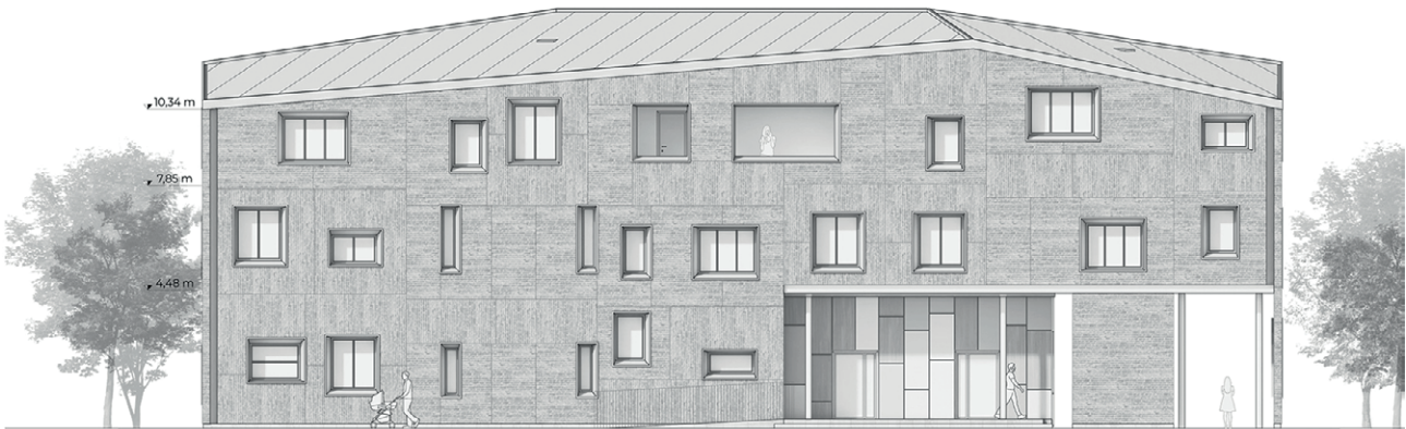
Figure 8 | Example of the reuse of existing external walls 'in parts' to create new façades.
