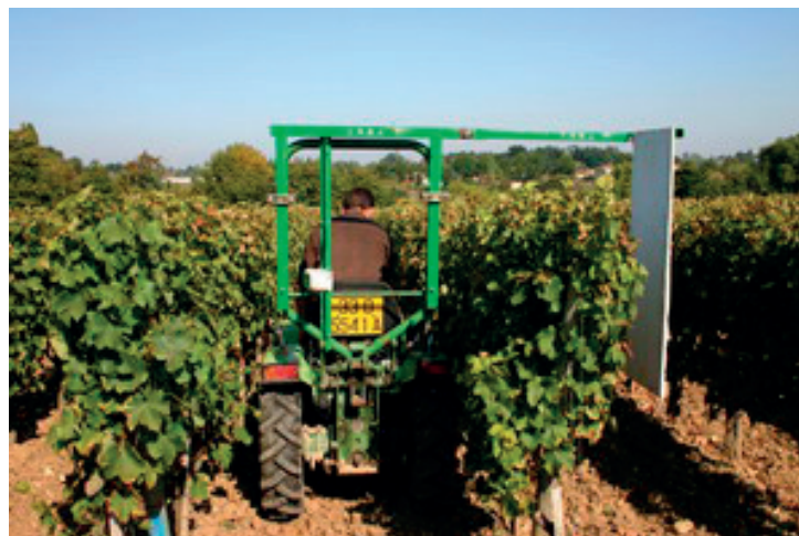
Figure 5 | The GreenSeeker (Avidor): measures vigour and estimates the optimum harvesting time. Source: www.cap-sciences.net
