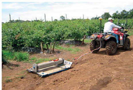
Figure 2 | b. EM-38 Geonic. Source: www.lb-track.cl
