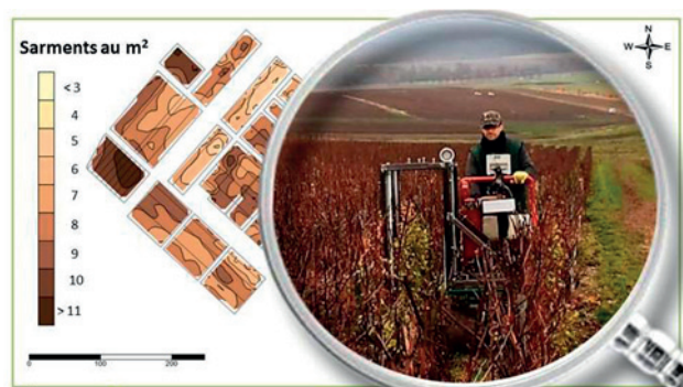
Figure 6 | Physiocap (Force A): pruning wood measurement and mapping (number of vine shoot, average wood diameter and wood biomass. Source: www.force-a.eu
