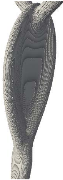
Figure 6. Close-up view of the collision of two jets with condition 2\alpha = 89^\circ , We = 58.8 , Re = 40.4 , u_j = 3.3 \frac{m}{s} .
