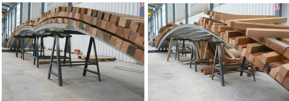
Figure 9: Arch failure by buckling.
