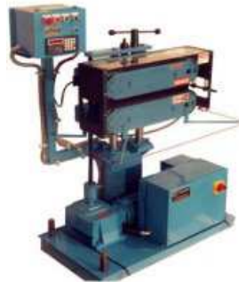
Figura 13: Arrastre tipo "oruga" [ http://www.scribd.com/doc/3901568/11-Extrusion ]
