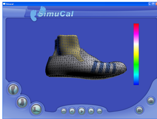
Figure 3.14: Meshes for the foot, for the shoe upper, and for the shoe sole.
