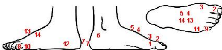
Figure 4.6: Distribution of the pressure sensors on the foot surface. Image from IBV.
