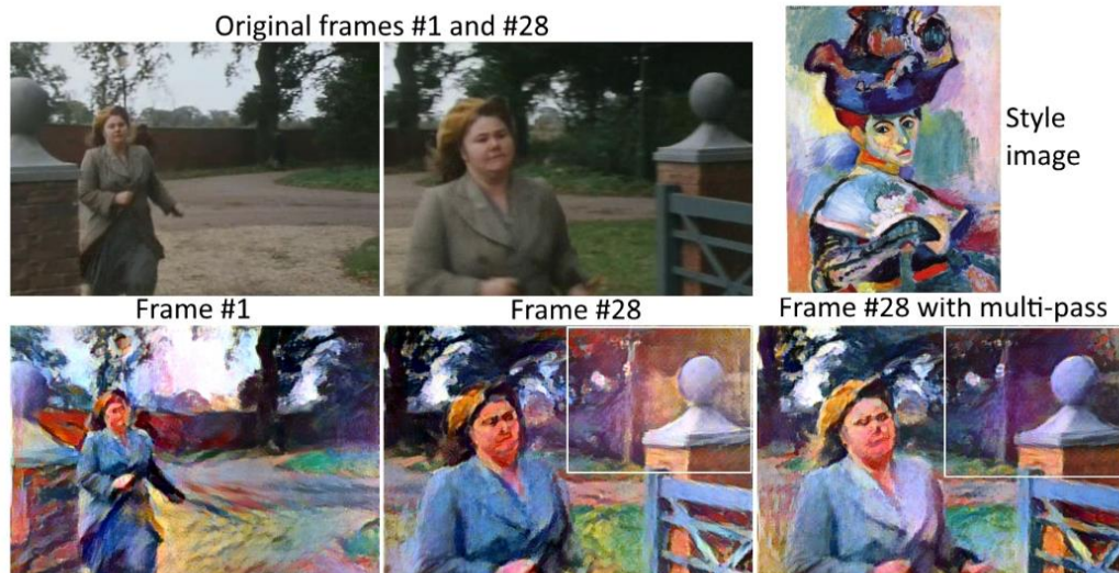
Fig. 40: The multi-pass algorithm applied to a scene from Miss Marple. With the default method, the image becomes notably brighter and loses contrast, while the multi-pass algorithm yields a more consistent image quality over time. Corresponding video is linked in section 8.1.
