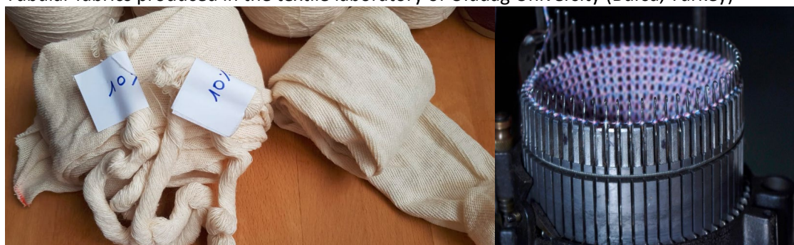
Figure 52 - Tubular knitting fabrics produced with the 3rd yarn sample. Figure 53 - Sample sock knitting machine.
