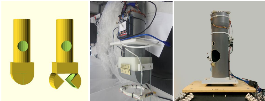
Figure 15. Object sequencer. (Left) the hatch at the bottom controls the fall of the objects; (Middle) the optical sensor that controls the trigger can be seen at the bottom; (Right) the sequencer prototype installed on top of the system, with the entry opening visible.
