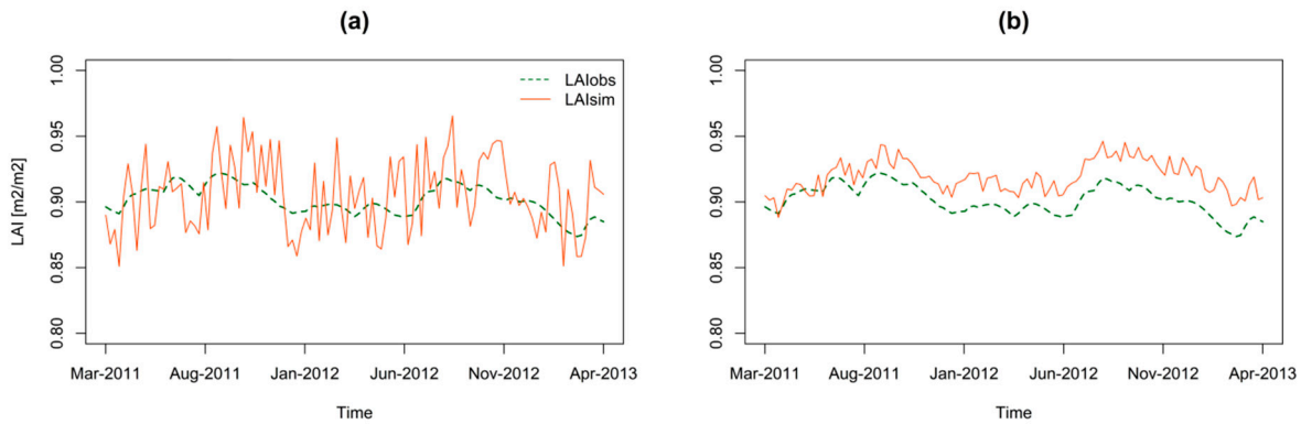
Figure 6. Observed and simulated mean area LAI during the calibration period (2011–2013) for: (a) streamflow-based configuration; (b) the SM-based configuration.
