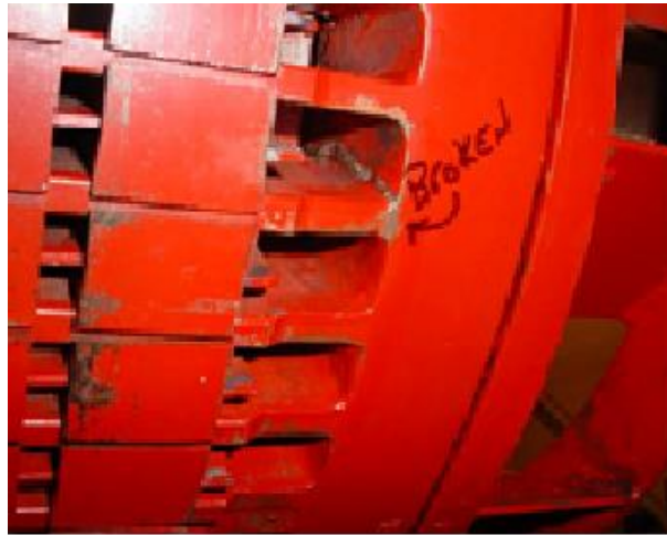
Figure 1. Rotor of a real industrial motor (2000 H.P) with broken rotor bars.
