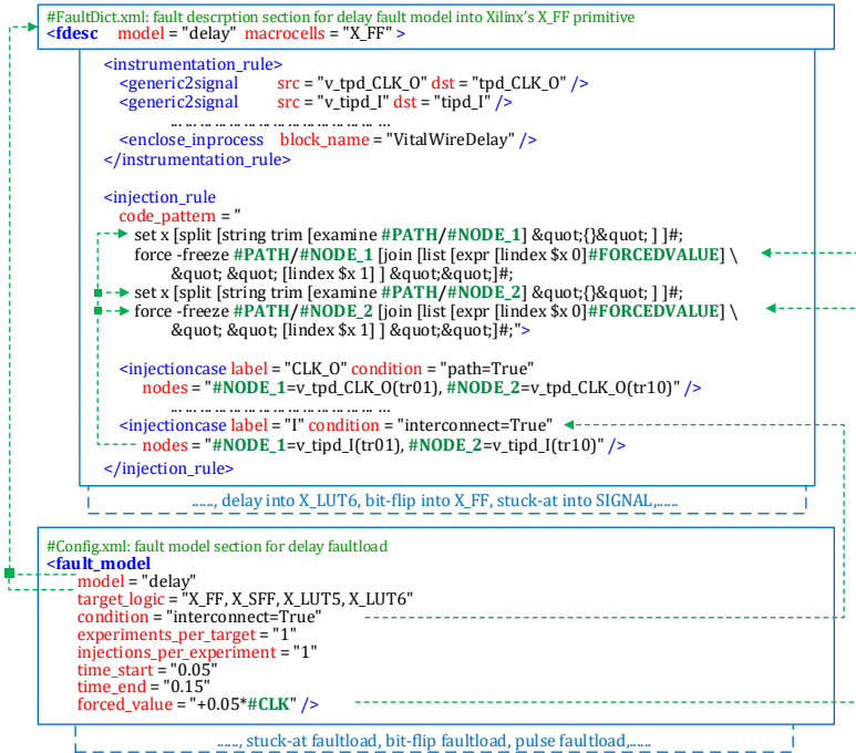
Figure 4.9: Excerpt from the fault dictionary file and configuration file describing the delay fault model for a Xilinx’s X_FF macrocells and a delay faultload, respectively
