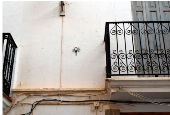
Figure 1. View of the datalogger on the outer surface of the rammed earth wall. Source: L. Balaguer.
