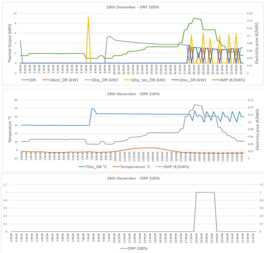
Fig 26: a) Heating system on 28 th December – DRP-100%; b) TES behaviour on 28 th December – DRP-100%; c) DRP-100%.
