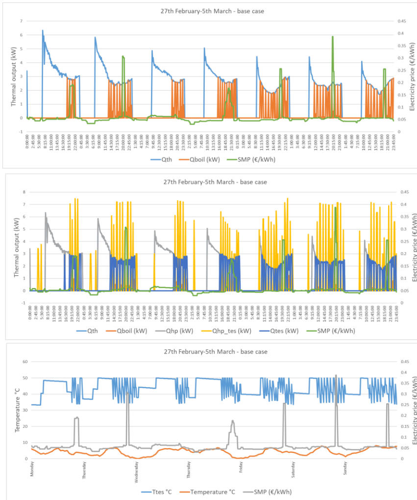
Fig 23: a) Gas boiler system on 27 th February-5 th March – Base case; b) HP system on 27 th February-5 th March – Base case; c) TES behaviour on 27 th February-5 th March – Base case
