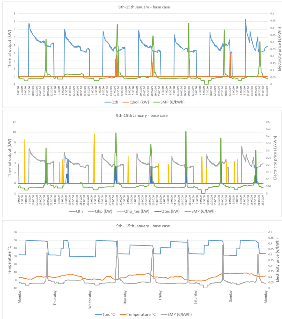
Fig 21: a) Gas boiler system on 9 th -15 th January – Base case; b) HP system on 9 th -15 th January – Base case; c) TES system on 9 th -15 th January – Base case.
