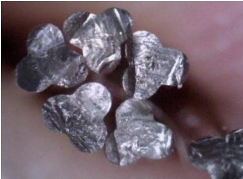
Figure 5. Photo of the cross-sections of the obtained plastic optical fibers.
