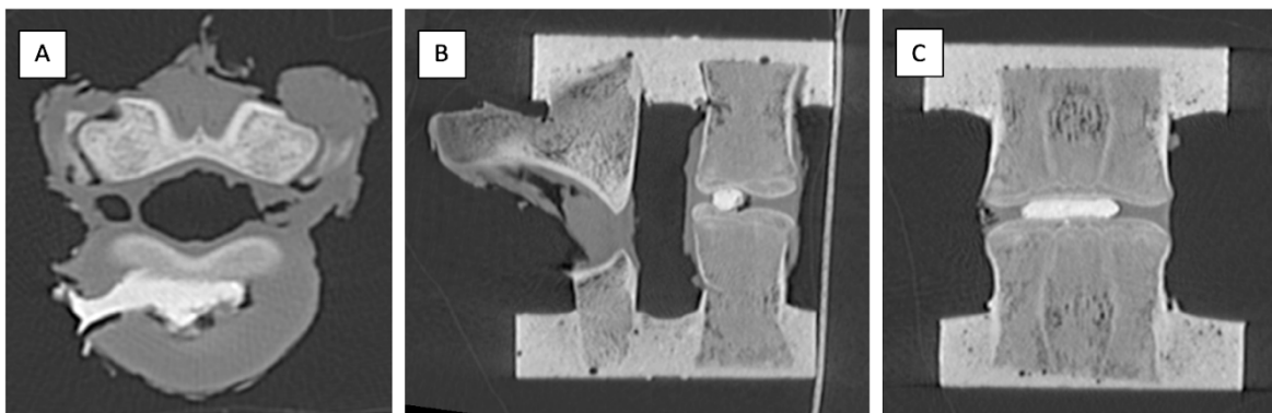
Figure 7. DICOM images of L3-L4 PMMA cemented specimen CT scanned. A: Axial view; B: Sagittal view; C: Coronal view.
