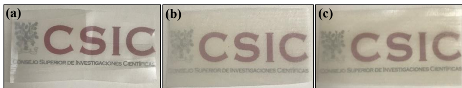
Figure 3. Visual aspect of: (a) YPACK210 film; (b) active multilayer films with cellulose nanocrystal (CNC) layers; (c) active multilayer films without cellulose nanocrystal (CNC) interlayer. Films are 5 cm × 2 cm.
