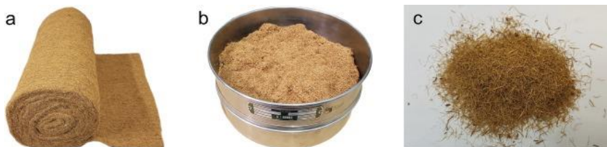
Figure 1. (a) As-received reel of coconut fibers (CFs); (b) Ground CFs; (c) Sieved CFs.
