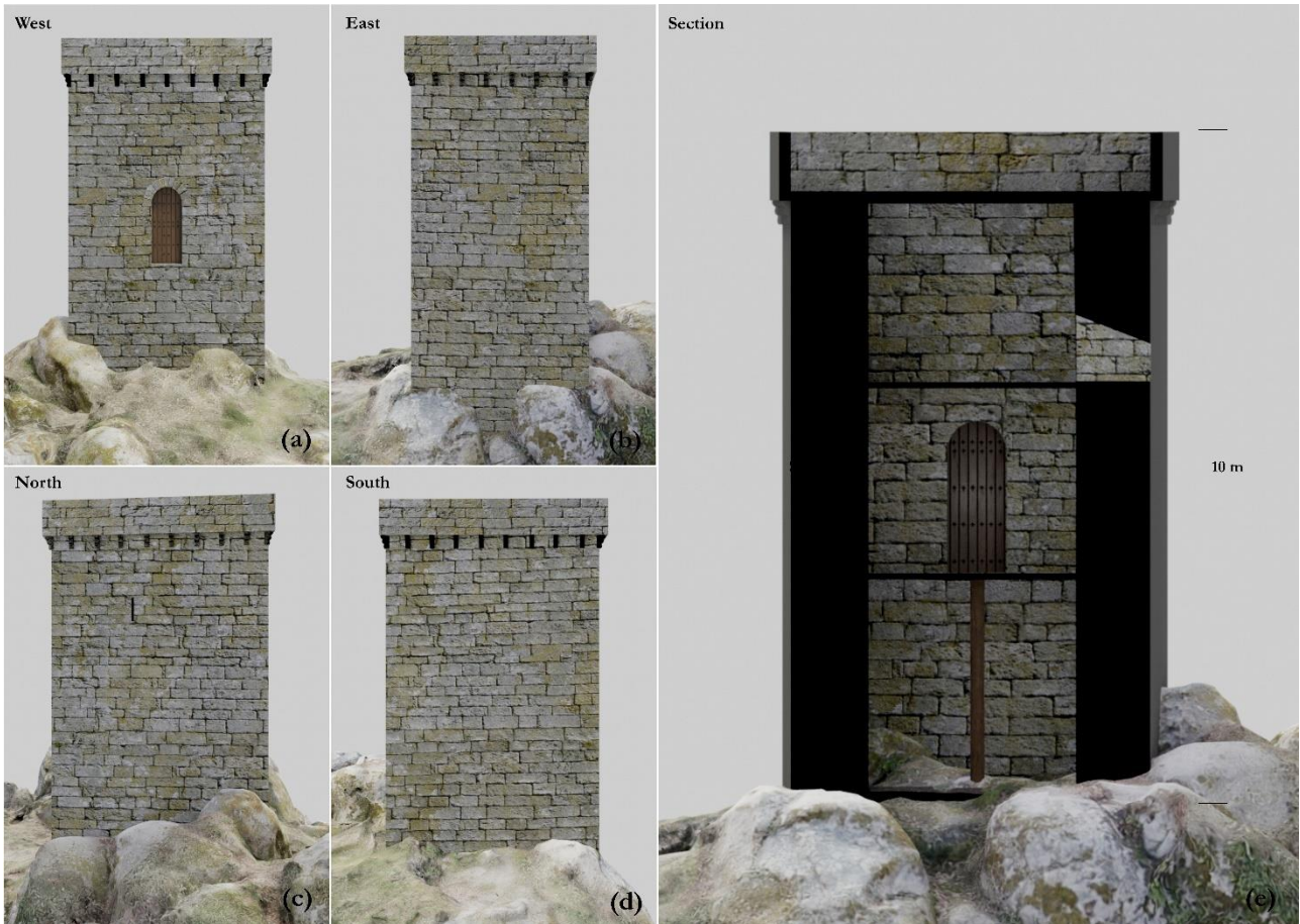
Figure 13: (a-d) Final aspect of the tower after its reconstruction and (e) hypothesis of its inner distribution. The possible entrance through the first floor and on the upper side the machicolation with reinforcements (a) were modeled following the aesthetic of other contemporary towers.
