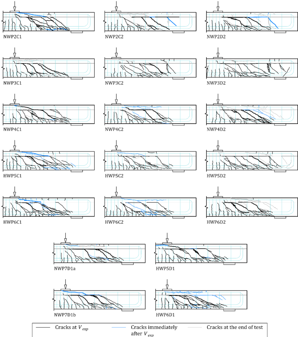
Fig. 8. Crack patterns of the test specimens in different test stages.
