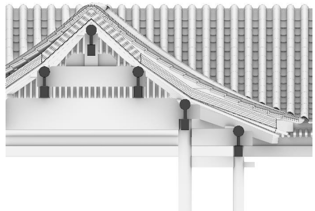
Figure 21: Section of the roof.
