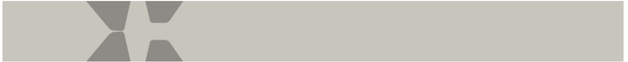
Figure 4: Computational domain for the phonation example with vocal folds in dark grey.
