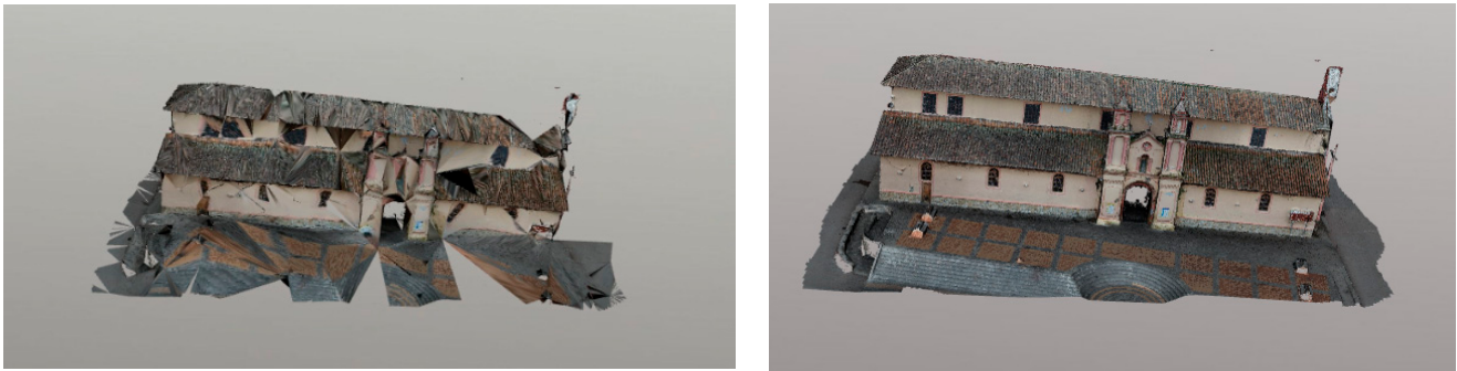
Figure 13. Multi-resolution 3D model of the Central Church of Nabón while uploading (left) and once complete (right).
