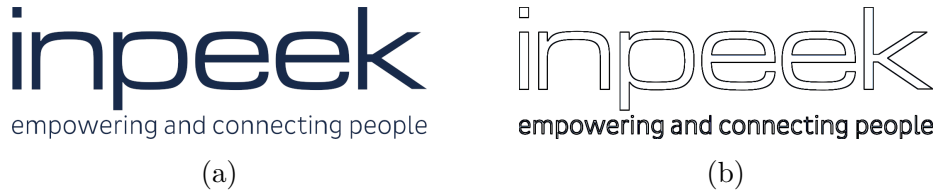
Figure 2: (a) Initial image and (b) the detection of borders with the convolution product.
