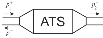
Figure 3.25: Nomenclature of pulses when an ATS is subject to an upstream excitation and with a non-reflecting downstream termination.
