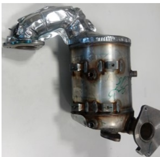
Figure 3.1: DOC-DPF Small bent pipes device.
