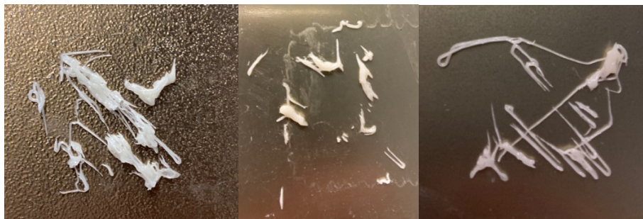
Figure 7-3: Influence of extrusion rate and retraction distance (Experiment 3), T_65_EM_1_ER_20_RD_1_; On the left side, repetition 1; In the center, repetition 2; On the right side, repetition 3
