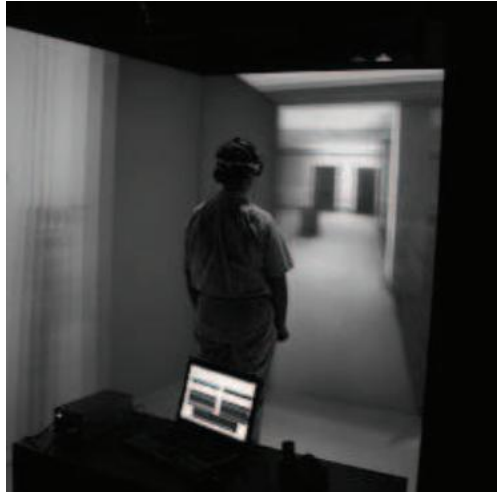
Figure 3.1 Photograph of a subject navigating through a virtual environment while the blood flow velocity is measured by TCD, from the study of Alcañiz et al. (2009)
