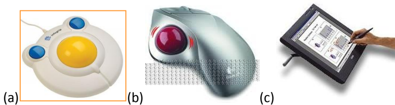
Figure 2.62 Examples of (a) a trackball, (b) a mouse and (c) a digital pad
