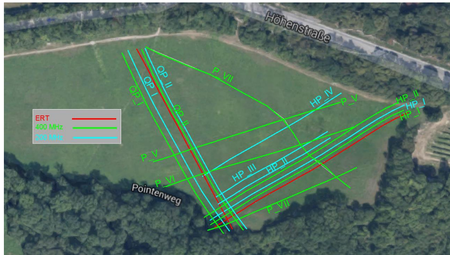
Figure 21. Disposition of ERT and GPR profiles in study area.
