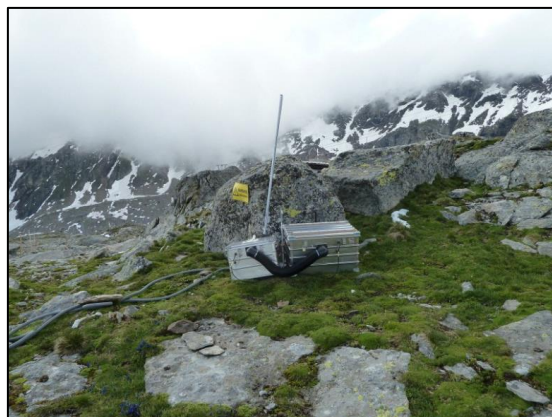
Figure 20. Image of Geotom multi-electrode equipment.
