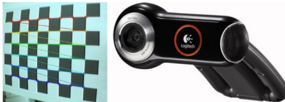
Figure 4.3: Checkerboard that is used to calibrate the camera. A Logitech QuickCam Pro 9000 webcam.
