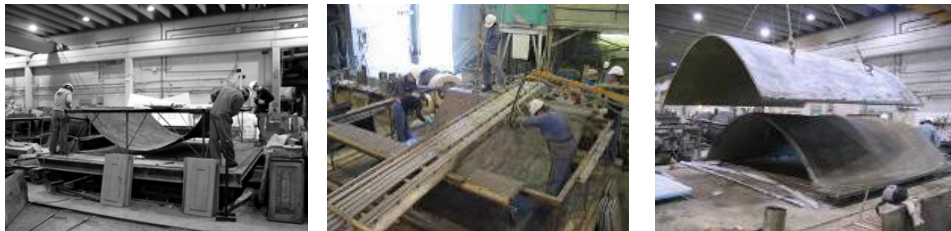
Figure 1 CAST's funicular fabric formed compression vaults
