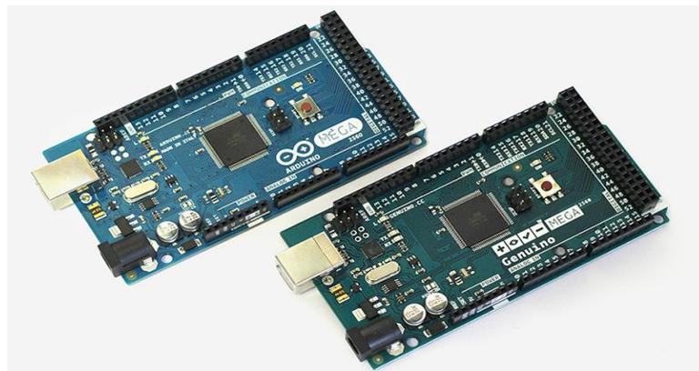
Figura 11: Arduino® Mega
