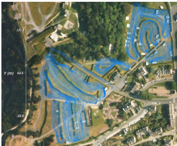
Figure 3: Area covered with the G.P Radar (doc. ABEM France).
