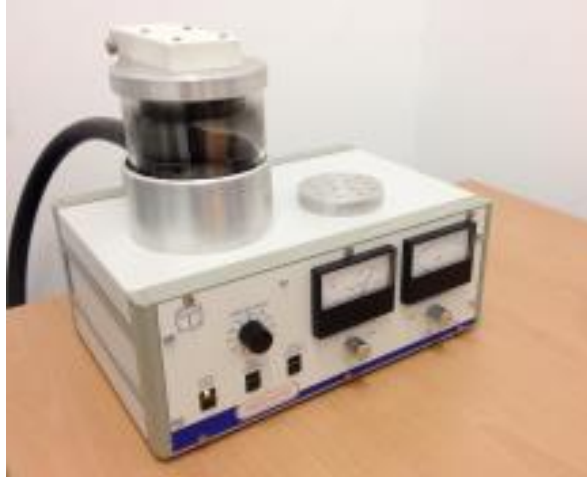
Figura 36. Sputter Coater EMITECH mod. SC7620
