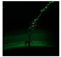
A) liquid injection in square hole's root (1000 rpm-10 LPH)
