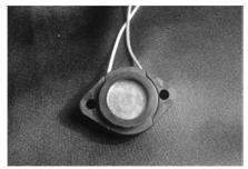
Figure 1. Image of one of the piezoceramic disks used in the present experiments
