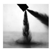
Figure 1. GDI spray impinging upon a smooth plate. Fuel pressure is 100bar.
