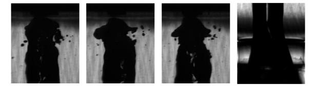
Figure 5. Simplex, p-cymene, Re = 1021. The detail on fluctuating end of the air core. Right: the detail on the exit orifice.
