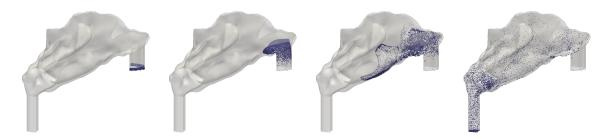
Figure 7. Temporal evolution of the particles of diameter 2.4  $\mu$ m for the pulsating airflow from left to right at t = 0.00555 s, t = 0.0222 s, t = 0.0555 s, and t = 0.333 s
