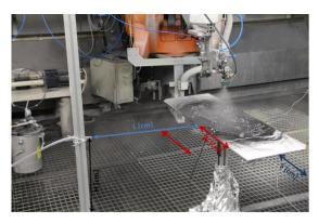
**Figure 5**. Setup of the spray application and sampling position definition.
