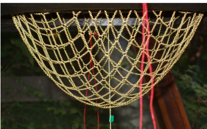
Fig. 7. Hanging chain net producing the antifunicular form of a grid shell supported all around its perimeter.
