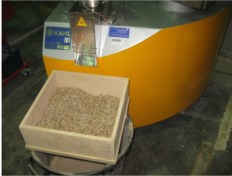
Figure 2a: Sample of experimental pellets manufactured with KAHL press with plane matrix of 50kg/h capacity
