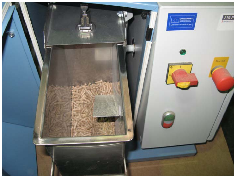
Figure 2b: Test of mechanical durability with Bioenergy TUMBLER Series following EN 15210-1
