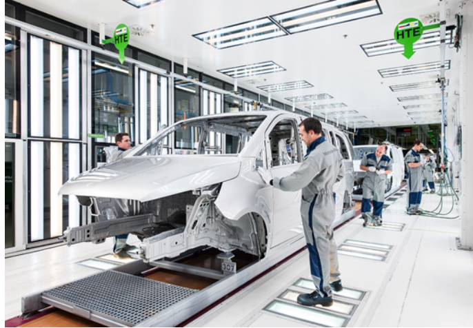
Figure 1: Check-men working on a production line, inspecting car body parts following the painting stage (image courtesy of Mercedes Benz España S.A.U., Vitoria Plant).
