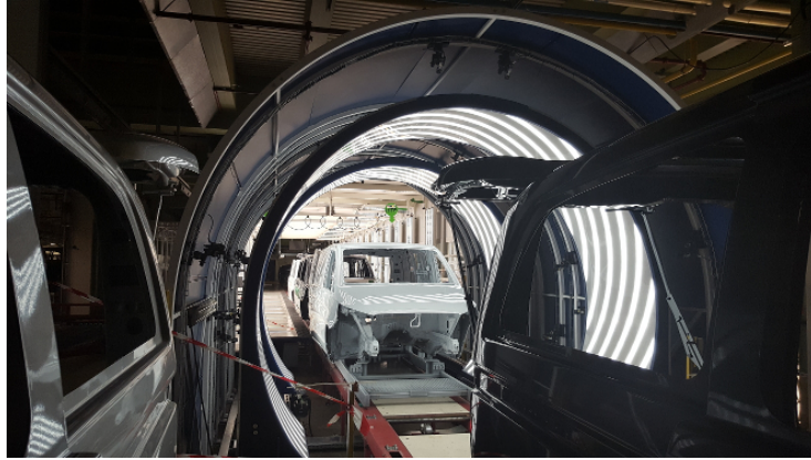
Figure 13: QEye-Tunnel : an Automated inspection system for surface body-car quality control based on artificial vision.
