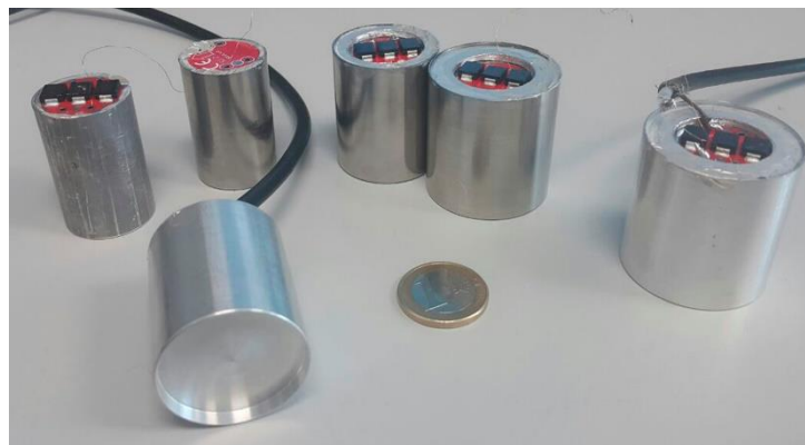
Figure 7. Three aluminum and three stainless steel sensors with 0.3 mm front-plate thickness and radius: 11.5, 15, and 17.5 mm. Each device is supported by a cylindrical structure 1.0 mm thick and 40.0 mm long. The ceramic material used in each device is PI Ceramics 255 with a 10.0 mm radius and 0.3 mm thick.
