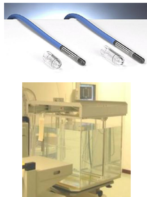
Fig. 6. Semiflex Chambers 31010 and 31013 and water phantom.
