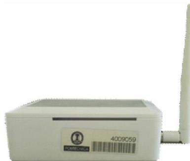
Fig. 1. Raspberry-pi Wi-Fi sensors
