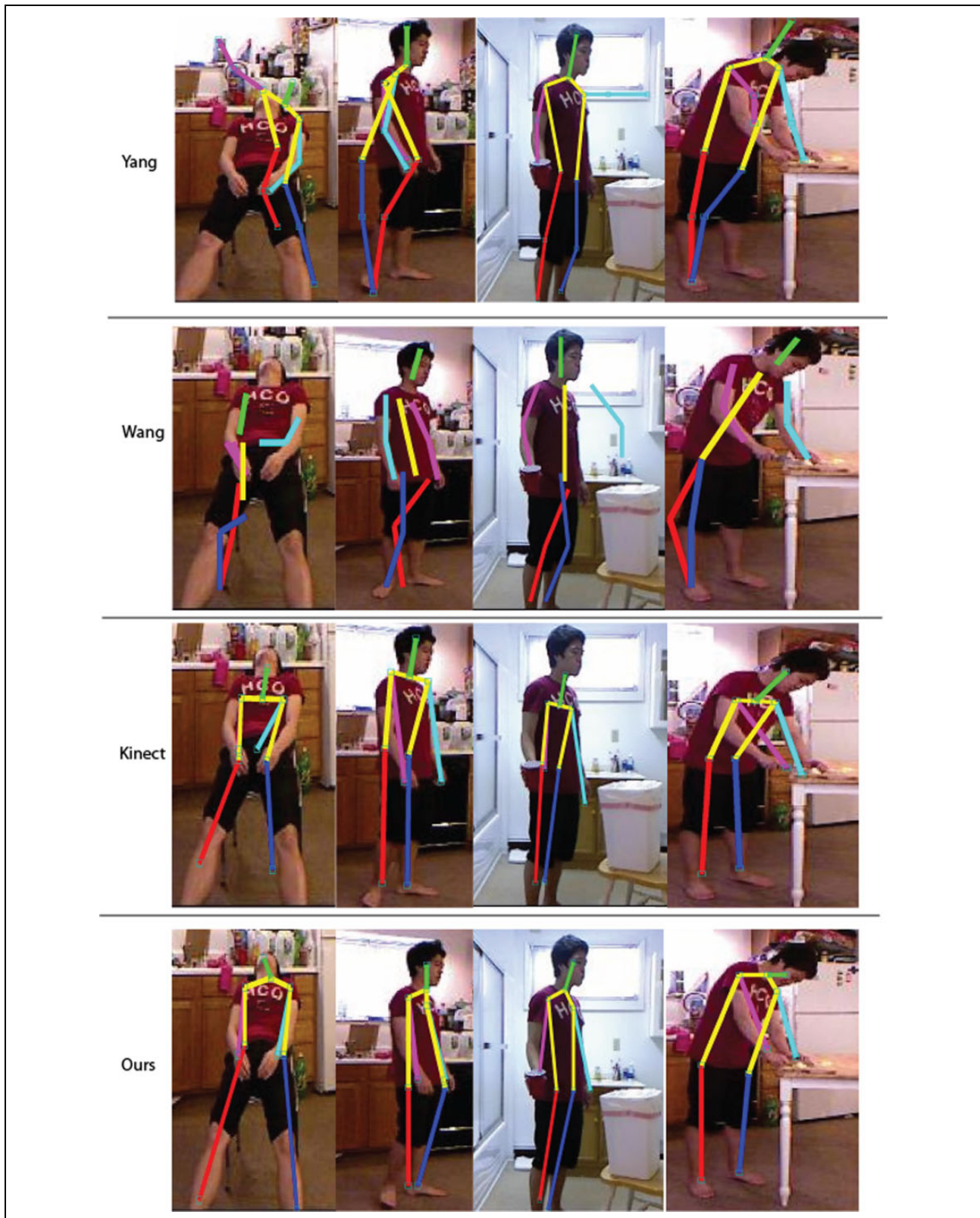
Figure 7. Qualitative comparison of four different methods for pose estimation on four sequences which belong to CAD60 data set. Fourth row shows joints of the reduced model.
